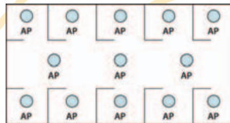
Figure 3B. AP configuration and density needed for RTLS.
